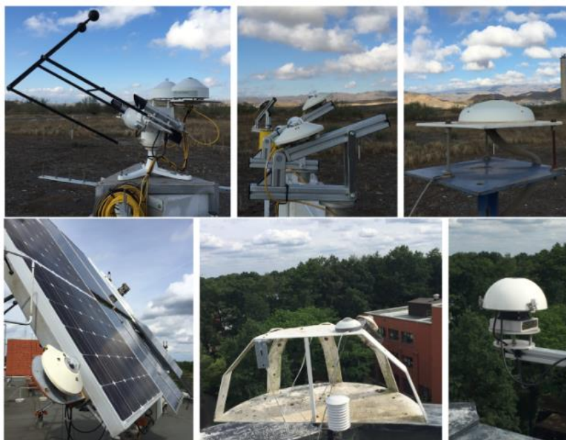
Figure 4 Setup at CIEMAT's PSA (top row): Solar tracker with pyrheliometer and shaded pyranometer (left), pyranometers in 3 tilted planes (center) and ASI (right). The pyranometer
