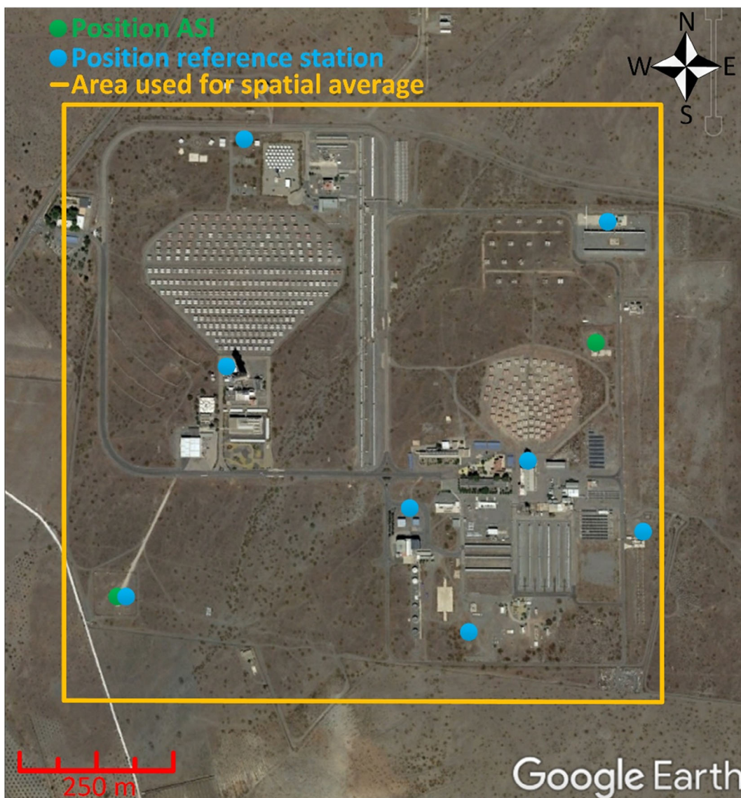
Figure 5. Aerial image of CIEMAT's PSA with markers for ASIs, ground-based irradiance reference stations as well as the area used for spatial averages (Source: Google Earth © 2021 Google. [Accessed: 25.05.2021]).
